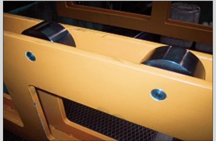
Stor rulldiameter minskar yttrycket Large diameter rolls that reduce specific pressure Grosse Rollendurchmesser vermindern Flächen Druck
